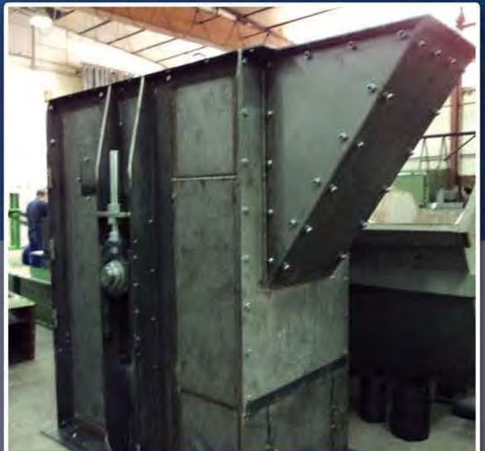
MANUFACTURING ELEVATOR FOOT
